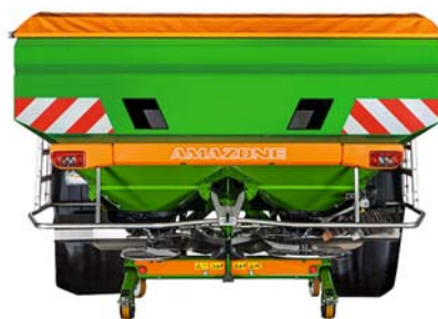
L 4200 extension (filling width 2.71 m) with foldable ladders
